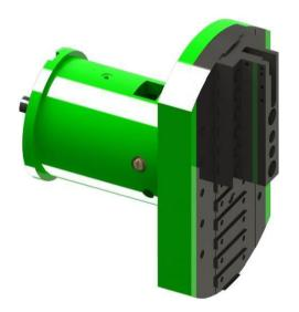
The VWD 500 / 630 Facing Head is attached to the hollow spindle of horizontal boring machines. The Facing head is identical for all types of the machines with exception of the mount and the taper shank. Movement of the tool position is carried out by the digital read out, feed of the slide is selected from the panel of the machine.
