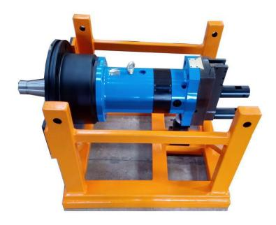
The VWD 320 Facing Head is attached to the hollow spindle of horizontal boring machines. The Facing head is identical for all types of the machines with exception of the mount and the taper shank. Movement of the tool position is carried out by the digital read out, feed of the slide is selected from the panel of the machine.
