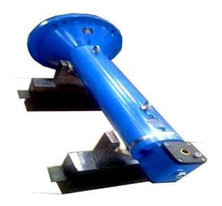
The VFW 1 Milling head is applied for light milling operations on small surfaces or for milling both external and internal slots which parallel with main spindle axis. It is also suitable for drilling small holes and, with special tools, for other operations such as production of internal clutch claws, internal splines and similar.
