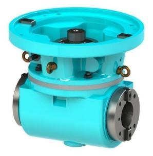
The VFH 3 duplex Milling head is applied for milling several faces which are parallel with the main spindle axis. The spindle of this head is fitted with taper at either end for clamping the cutters. The head may be swivelled through 0-360° by an worm and worm gear arrangement at required position.
